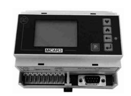
The MCAR3 is a communication module for data transfer from an AR3DC system to a control computer. It has two serial communication lines, one dedicated to the instruments and the other for the computer connection.
